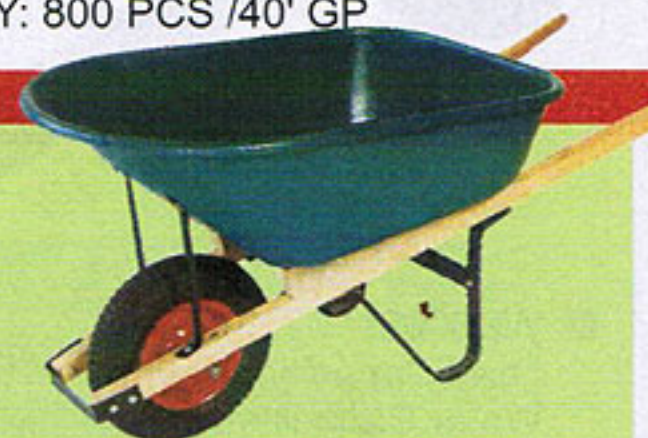
WB5005 Load Capacity(kg):150 Water Capacity(L):75 Sand Capacity(CBF):4.5 Wheel: 16 " × 4.00-8 Air L/H/C/A/B/h: 1530×442×560×855×600×280 QTY: 800 PCS /40' GP
